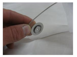
• Insert the screw into the aluminium disc and then hold the Mylar washer on the inner face of the visor.
