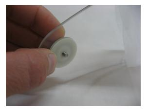
• Holding the aluminium disc and the Mylar washer in position in the hole in the visor, place the screw into the threaded bush of the helmet, and screw it down, using the hexagonal key provided.
