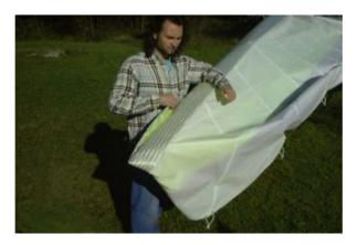
• Keeping the extreme part of the sail in this position, take the sail by the trailing edge and raise it upwards until it is tight and from this position roll up the sail starting from the trailing edge.
