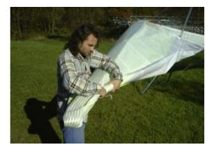
• Holding the rolled sail, slip the tip-bag over the tip.
