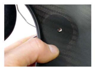
Place the steel washer onto the hollow bolt, and then insert the hex drive screw.
