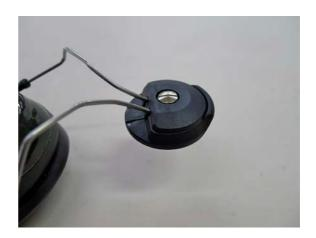
• Then place the earphone onto the helmet, so that the hollow bolt enters the hole on the helmet shell.
